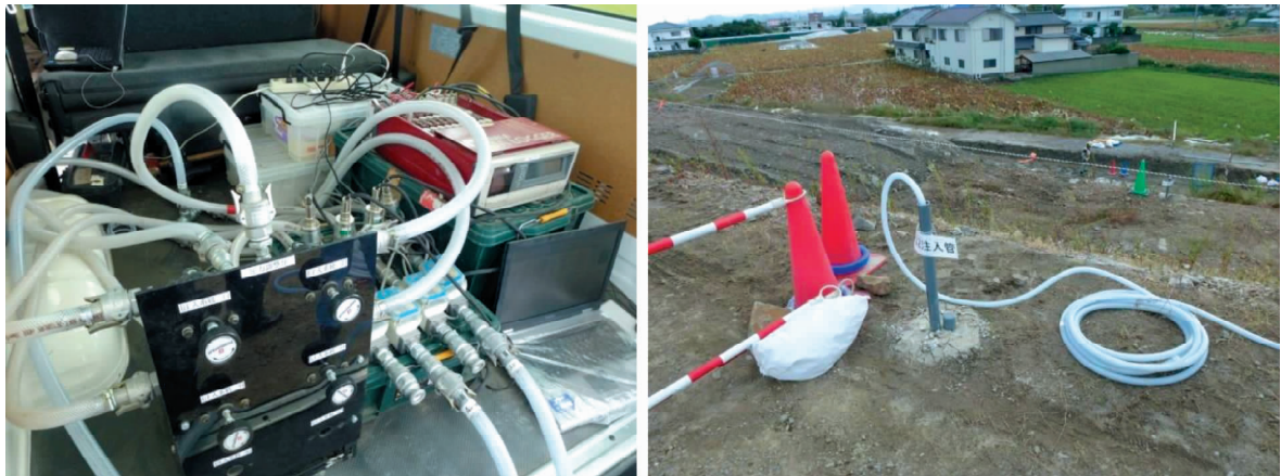
Figure 5. Air injection system at the site
