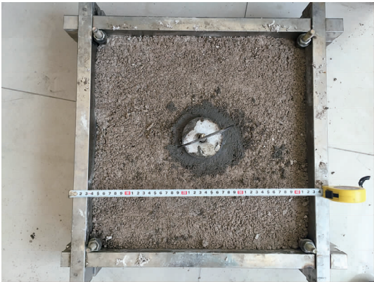
图 3 巷道模型养护 Fig. 3 Model of roadway maintenance
