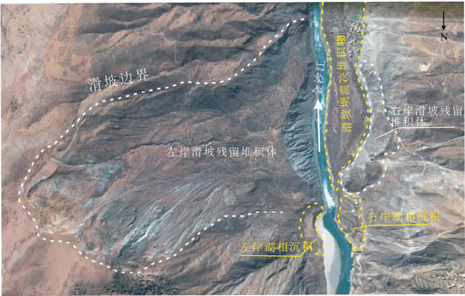
图 3 湖相沉积、特米滑坡和滑坡坝溃决堆积物的空间位置分布 Fig. 3 Spatial distribution of lacustrine deposits and accumulation masses of Temi landslide and landslide dam outburst deposits
