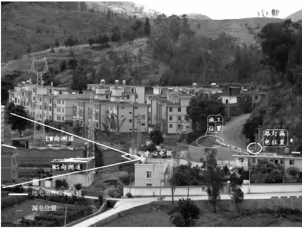
图 7 弥渡地电场测区环境及漏电路灯位置图 Fig. 7 Environment around geoelectric field measuring area at Midu Station and the location of street lights with leakage
